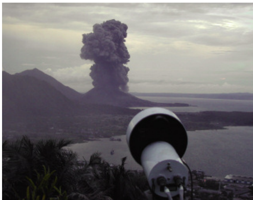
The volcanic ash detector monitoring volcanic eruptions from Tavurvur volcano at Rabaul, New Britain, in Papua New Guinea.
