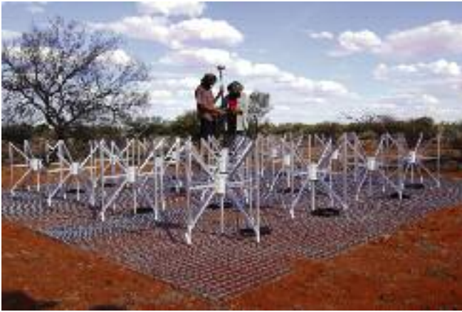
David Herne (left) and Mervyn Lynch of Curtin University of Technology at the Murchison Radio-astronomy Observatory deploying tiles for the Murchison Widefield Array (MWA) telescope, a forerunner of technology for the SKA. Photo: Dragonfly Media
