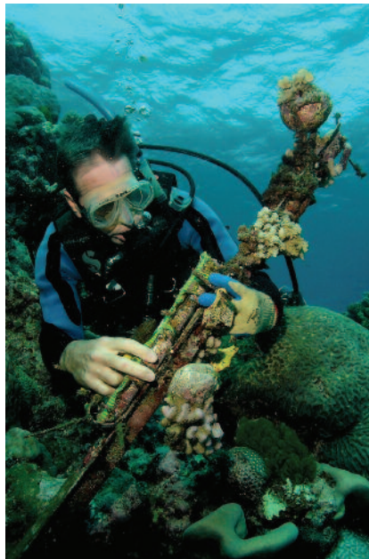
Dr Ray Berkelmans changing a temperature logger as part of measurements of the effect of temperature on coral growth.
