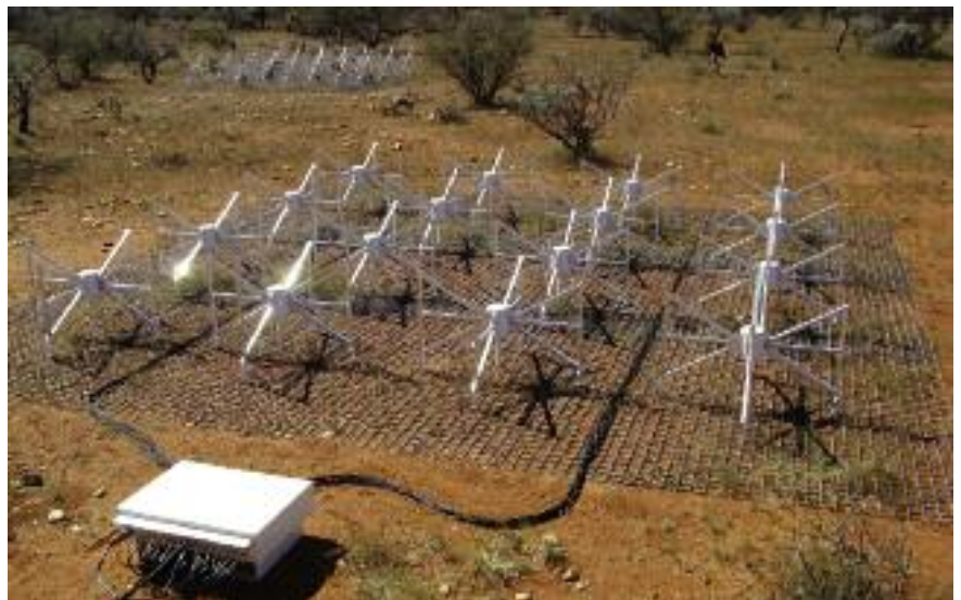
Figure 3. Antennae tiles making up the prototype MWA. Each tile consists of 16 cross-dipoles on a square grid. When complete, the full MWA will comprise 500 antenna tiles distributed over an area of diameter 1.5 km. The beam-forming box that will be used to electronically steer the array can be seen in the foreground. Image: David Herne, Curtin University
