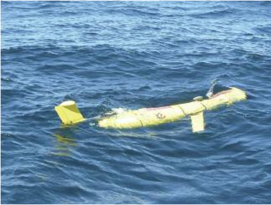
Slocum glider 2 after its launch into the East Australian Current off Crowdy Head south of Port Macquarie, NSW, on 17 March 2009. The communication link to the Iridium satellite network sits on top of the tail. Photo: courtesy Iain Suthers
