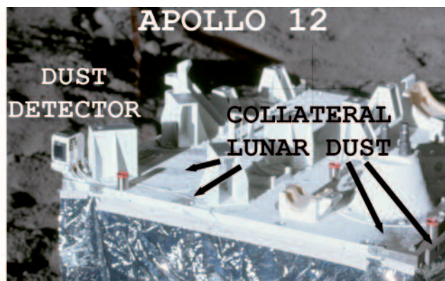
Sticky lunar dust accumulated on instruments deployed during the Apollo missions.
